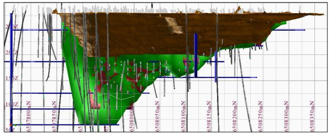
Figure 1-1. Long Section and Plan of Mt Boppy with drilling
