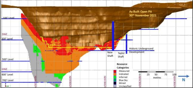
Figure Error! No text of specified style in document.. Long Section: Resource Classification
