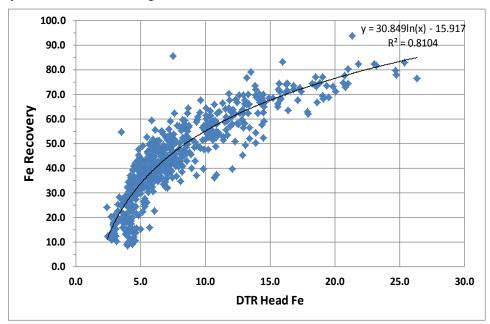
Figure 7-4 DTR Fe Recovery vs. Fe Head Grade
