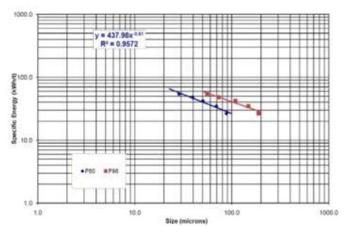
Figure 7-16 Signature Plot – First Stage Grind
