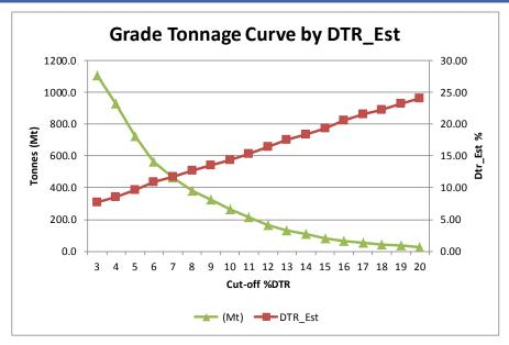
Figure 5-3 Grade Tonnage Curve - Based on DTR\_Est%
