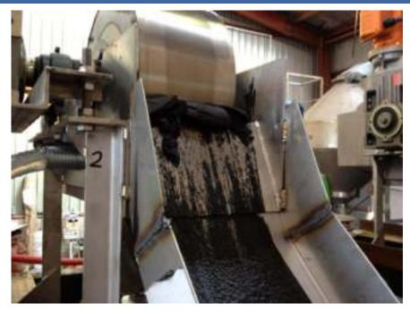
Figure 7-9 Pilot Plant LIMS-1 Concentrate
