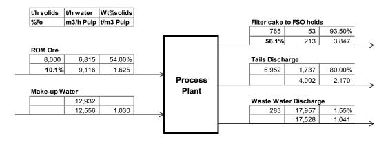
Figure 7-18 Process Plant High Level Mass and Water Balance
