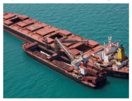
Figure 10-3 Gravity Transhipment Shuttle Vessel CSL Whyalla transhipping iron ore in South Australia
