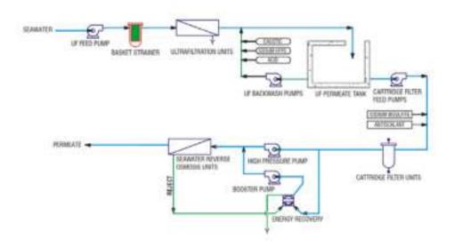
**Figure 8-4 Typical Desalination Process**
