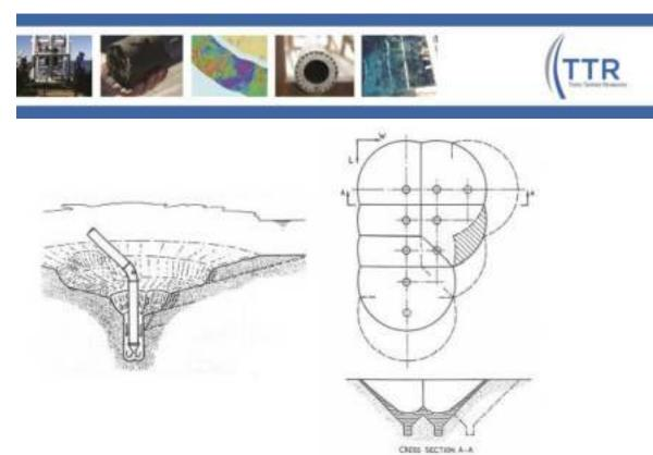
Figure 6-5 Suction pit geometry
