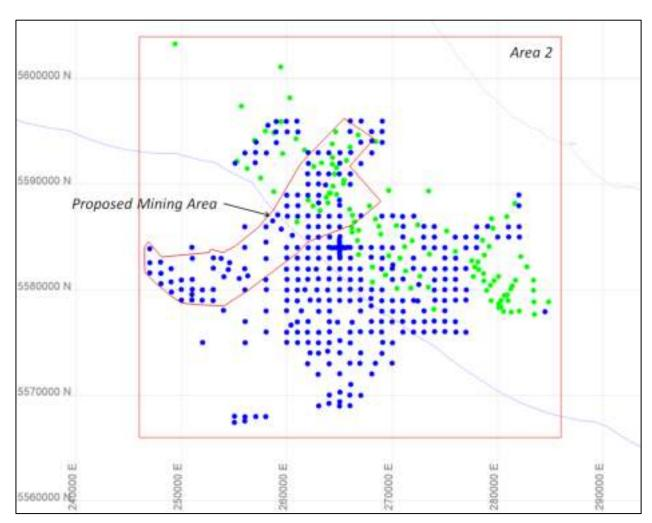
Figure 4-20Drill Holes in the Proposed Mining Area
