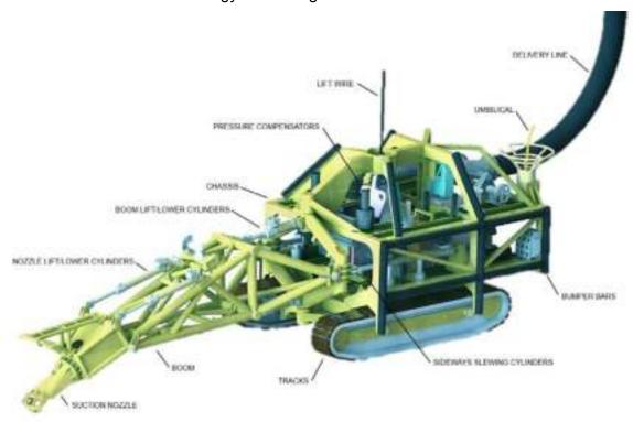
Figure 3-3 Subsea Sediment Extraction Device
