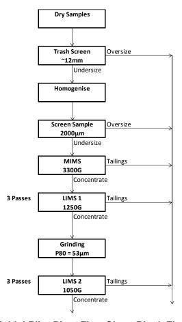
Figure 7-7 Initial Pilot Plant Flow Sheet Block Flow Diagram
