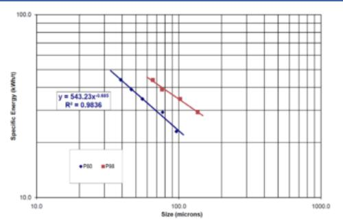
Figure 7-17 Signature Plot – Second Stage Grind
