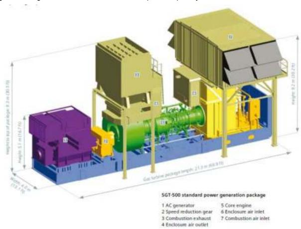
Figure 8-1 SGT-500 Power Generation Package
