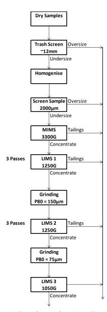
Figure 7-11 Two Stage Grinding Flow Sheet
