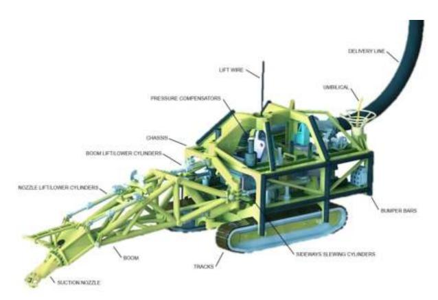
Figure 6-1 Submerged Sediment Extraction Device
