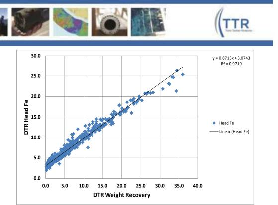
Figure 7-3: DTR Head Fe vs. Weight Recovery
