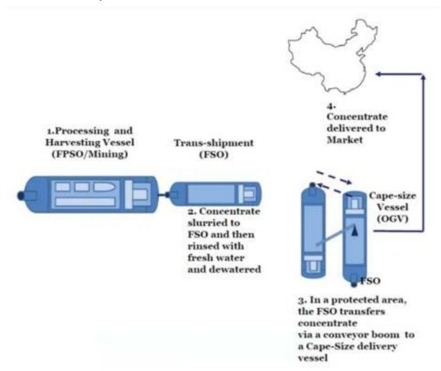
Figure 3-2 Offshore Operations
