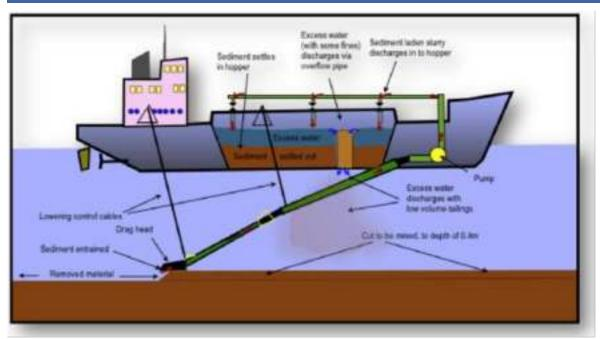
Figure 6-6 Typical section of the TSHD
