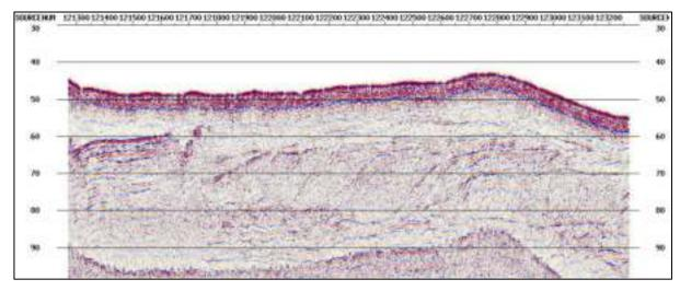
Figure 4-13Processed seismic line 107 profile showing sub-surface infilling of a paleochannel
