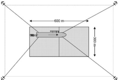
Figure 10-2 Anchor Spread
