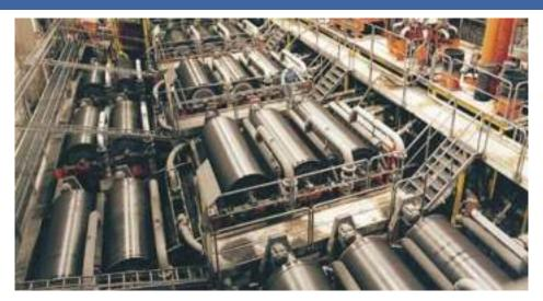
Figure 7-23 Triple and Double Drum Magnetic Separators
