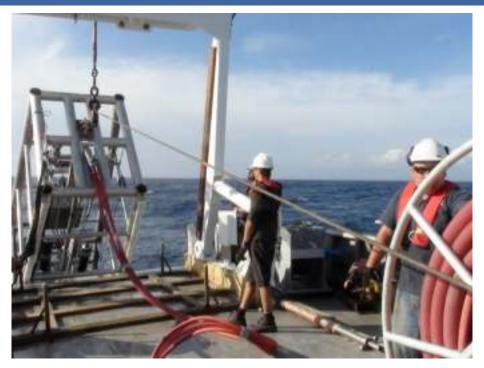
Figure 4-8Launching of the 11m shallow drill rig from the Island Leader II (2011 shallow drilling programme)
