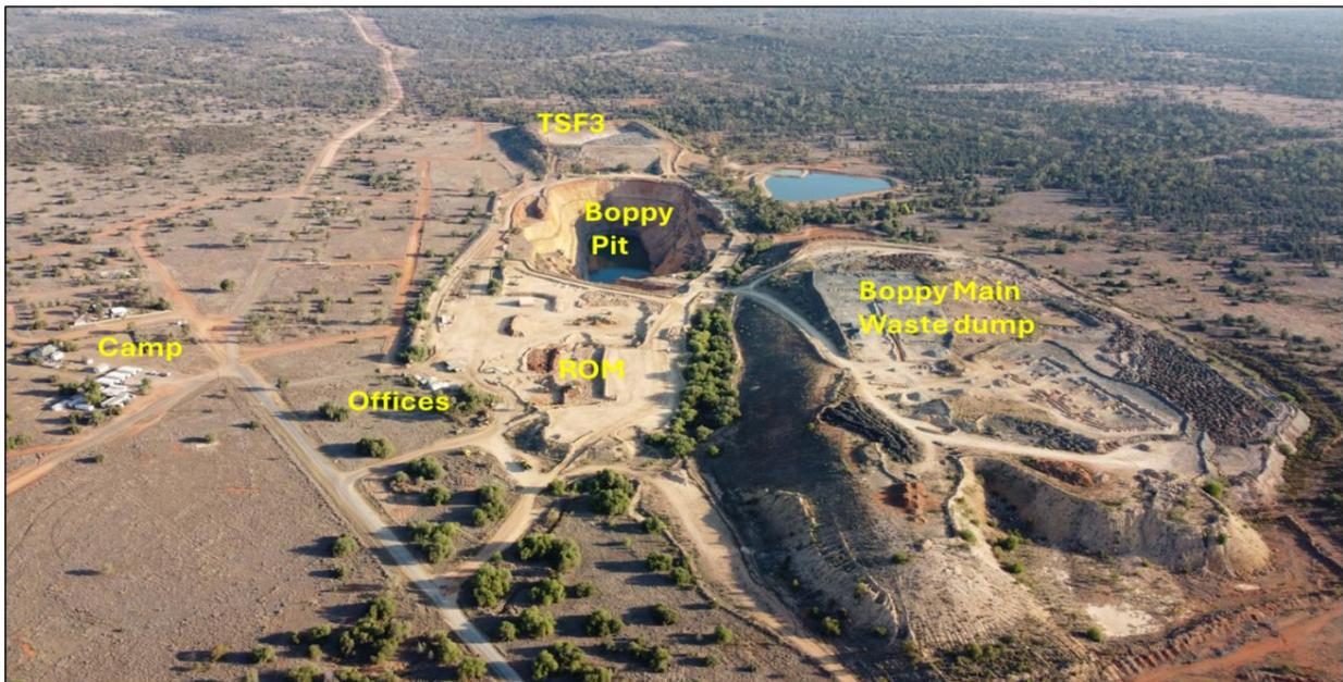
Figure 1: Drone image looking south showing the main components of the Rock Dump and Tailings Resources in relation to the Mt Boppy open pit.
