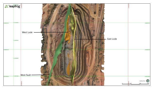
Figure 1. Plan of Boppy 3D model showing relationship of West Fault to lodes
