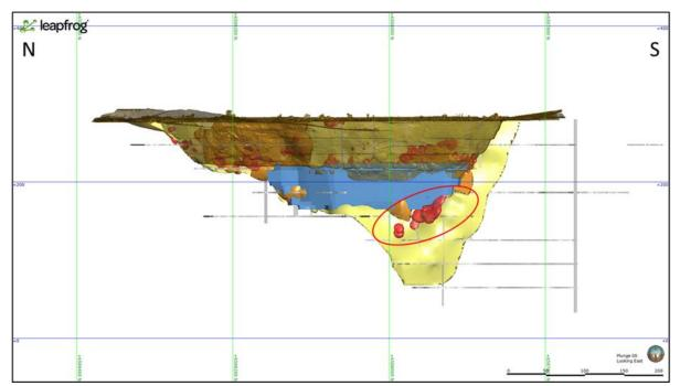
Figure 3. Long section looking east showing design pit (blue) and high-grade zone indicated by 5 g/t Au isosurface (red solid areas) generated in Leapfrog. High-grade target zone outlined by the eclipse.
