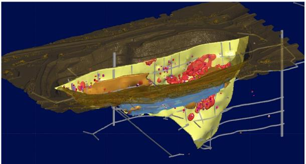
Figure 4. Long view looking east. illustrative separation of the west lode (in orange), east lode (in yellow) and current planned mine pit shell (blue), with high-grade zones extending below. Historical stopes visible.
