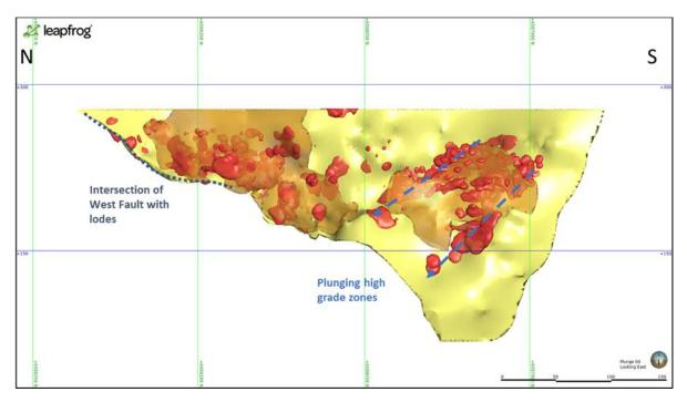
Figure 2. long section looking east showing north-plunging high-grade zones in southern part of deposit. Intersection of West Fault with lodes in north of deposit creates south plunge to mineralisation.
