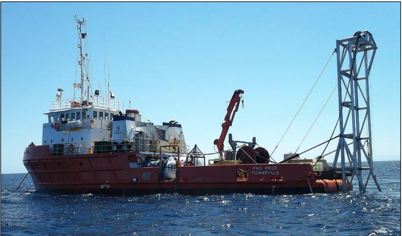
Figure 3-5: PMG Pride – Drill Rig Deployed
