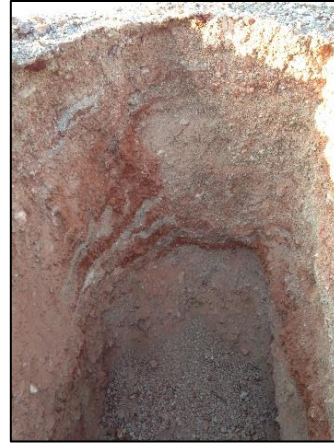
Photograph 4. Excavation in Clay Stockpile at Site CSP06.
