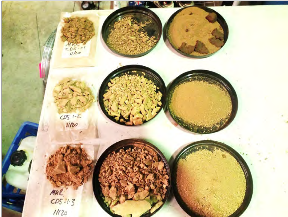
Photograph 4. The gravel content of natural ground to the east of WRE increased with depth generally being 10–20 % in topsoil, 40–60 % in upper subsoil and 40–80 % in lower subsoil.
