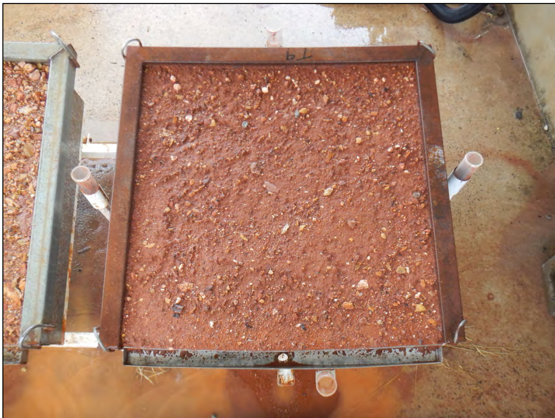
Photograph 14. Gravelly Topsoil test plot after receiving simulated rain at 125 mm/hr.
