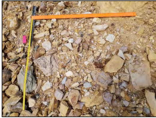
Photograph 13. Waste Rock Oxide material (Site WRO1) in an armored condition from rainfall.
