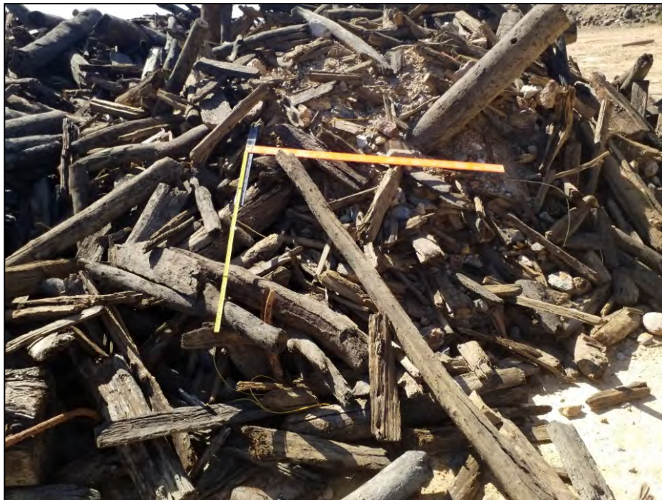
Photograph 23. Timber debris stockpile on the WRE. The log diameters generally range from 0.1-0.3 m. The 1m x 1m ruler is placed to indicate the scale of the stockpile.
