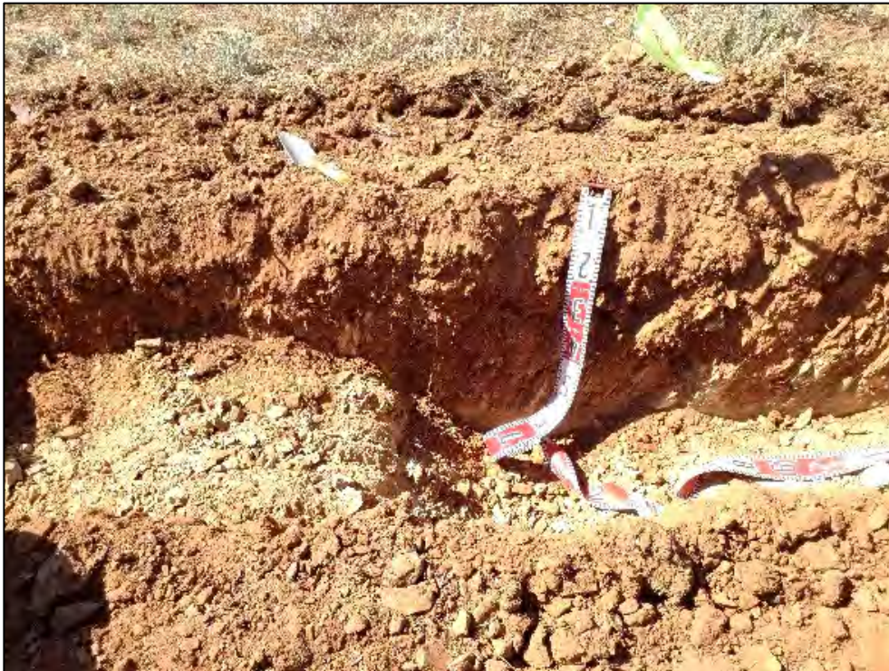
Photograph 3. Soil profile of natural ground to the west of WRE (Site CD5-01). Soil profiles in this area contained appreciable gravel content.
