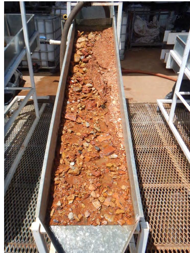
Photograph 20. Waste Rock Oxide plot tested to failure with overland flows.
