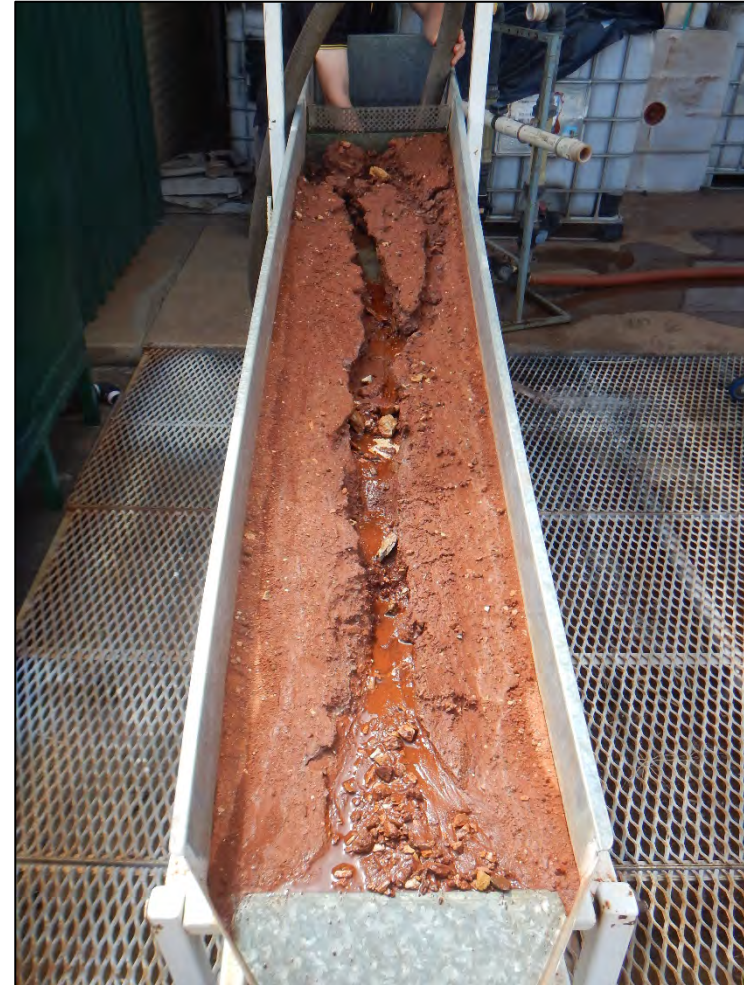
Photograph 18. Gravelly Topsoil plot tested to failure with overland flows.
