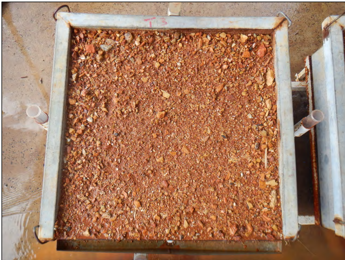
Photograph 16. Waste Rock Oxide test plot after receiving simulated rain at ~125 mm/hr..
