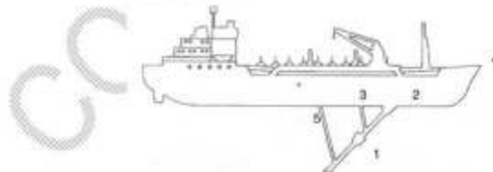
Figure 17: Typical TSHD. 1: Suction tube with drag head, 2: Dredge pumps, 3: Hopper, 4: Bow coupling, 5: Bottom doors
