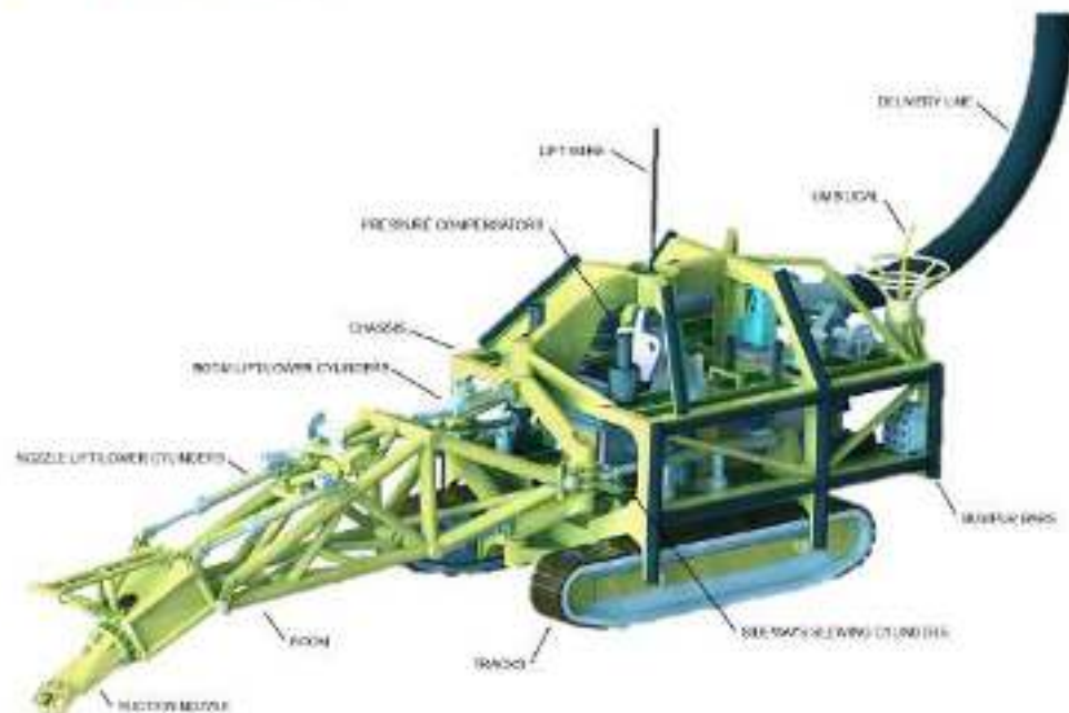
Figure 4-1: Seafloor mining tool (SMT) concept.
