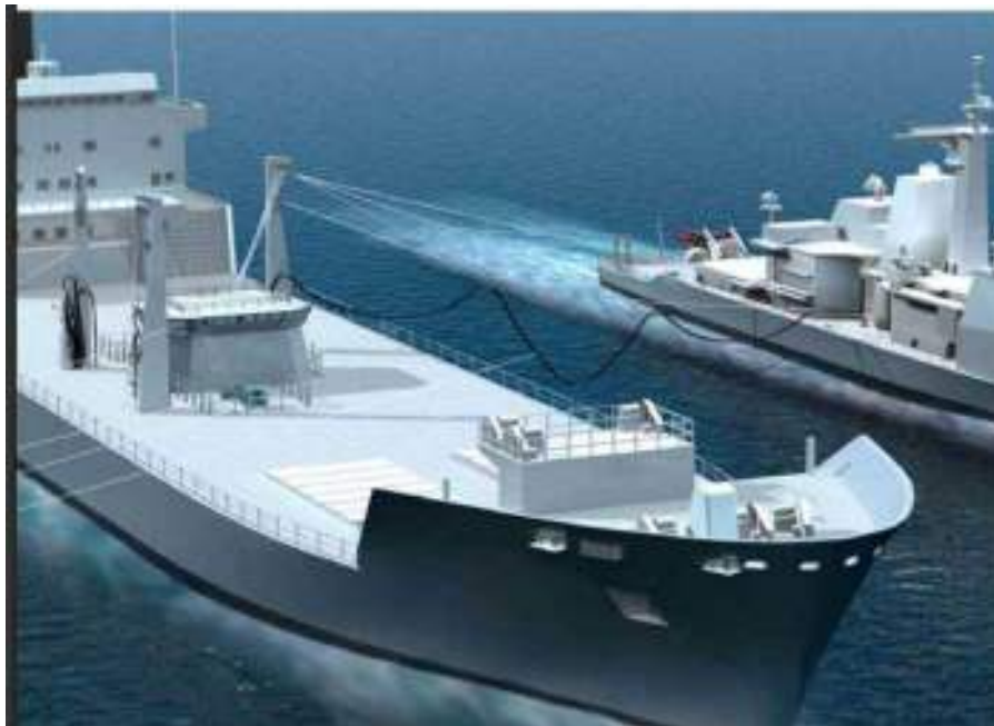
Figure 10-5 Typical Refuelling Configuration
