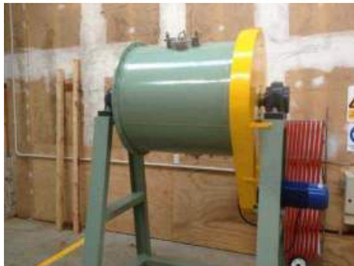
Figure 7-10 Pilot Plant Ball Mill
