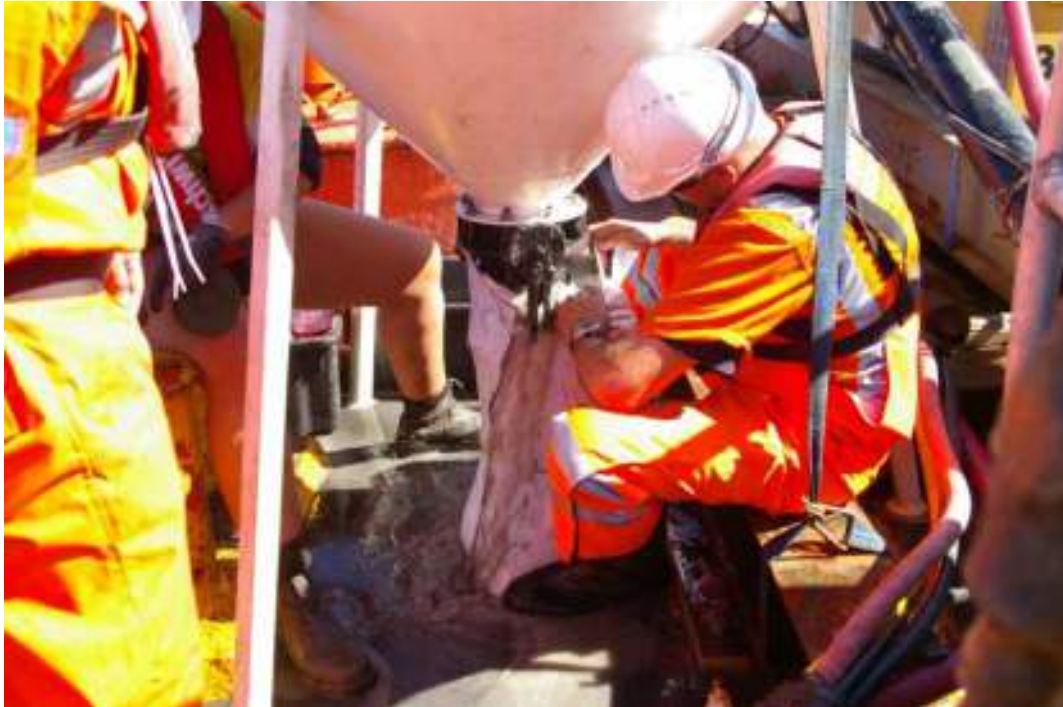
Figure 4-11 Collection of drill samples from deep drilling
