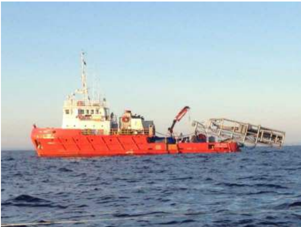
Figure 4-9 Deep drilling rig and LARS on the PMG Pride during the 2013 deep drilling programme.
