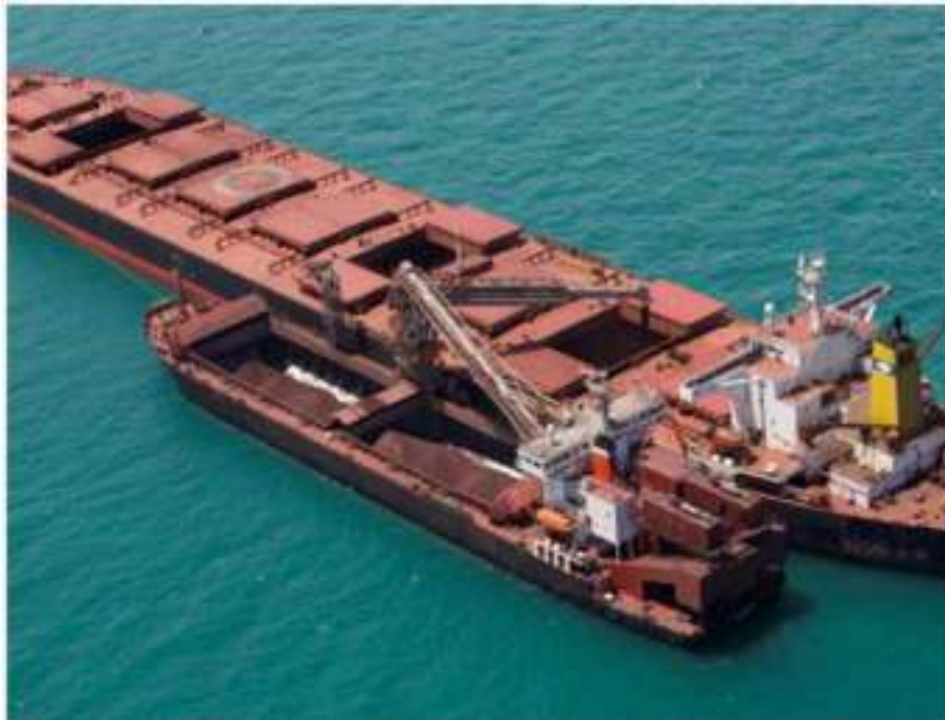
Figure 10-3 Gravity Transshipment Shuttle Vessel CSL Whyalla transshipping iron ore in South Australia
