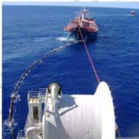
Figure 21: Aker-Pusnes off-loading solution using guide wire and reeled slurry pipe line. (source: http://www.akersolutions.com/ )
