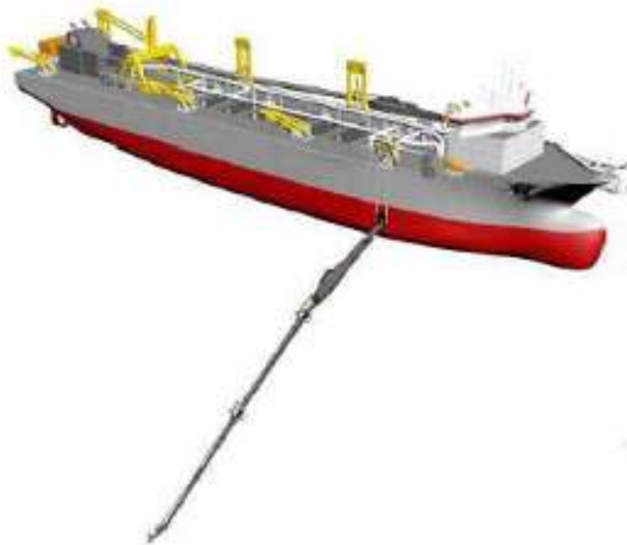
Figure 3: Trailer suction hopper dredge
