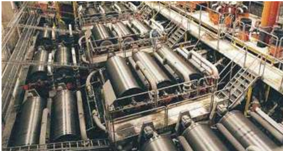
Figure 7-23 Triple and Double Drum Magnetic Separators
