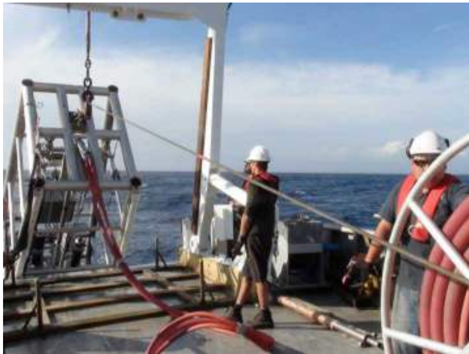
Figure 4-8 Launching of the 11m shallow drill rig from the Island Leader II (2011 shallow drilling programme)
