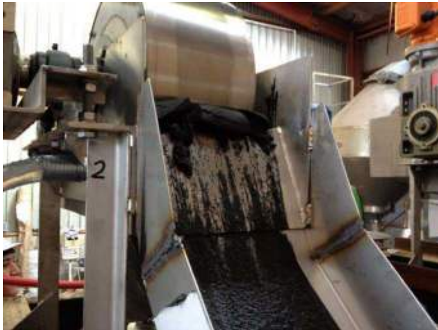
Figure 7-9 Pilot Plant LIMS-1 Concentrate
