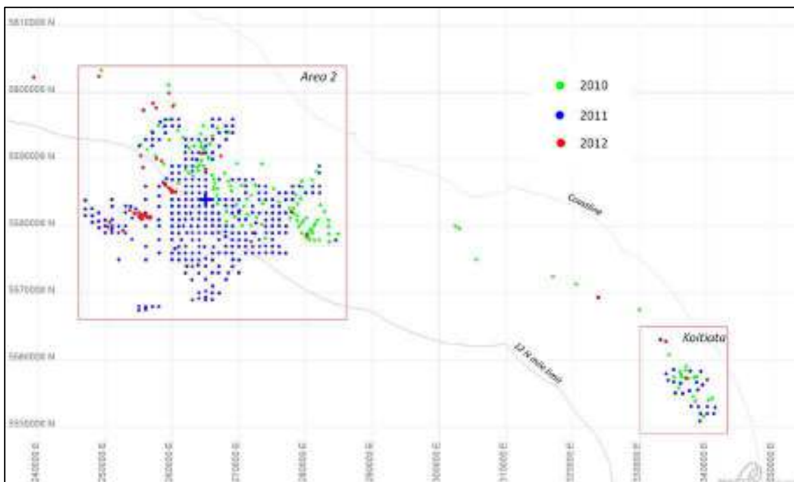
Figure 4-19 Drilling Locations - TTRs Iron sand Deposit
