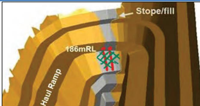
Figure 29-1 View looking south showing support for stope fill crossed by haul ramp at southern end of pit
