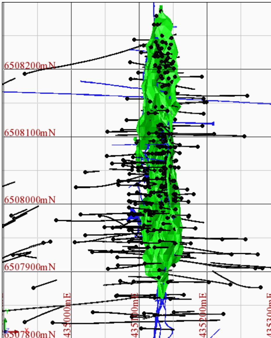
Figure 1-2: Mt Boppy Plan View showing mineralisation and drill hole locations
