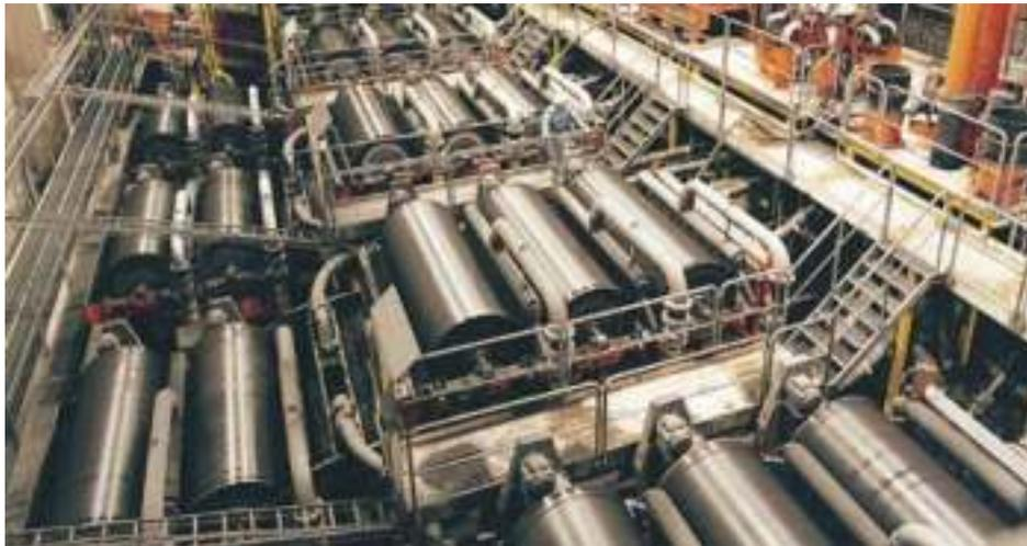
**Figure 7-23 Triple and Double Drum Magnetic Separators**
