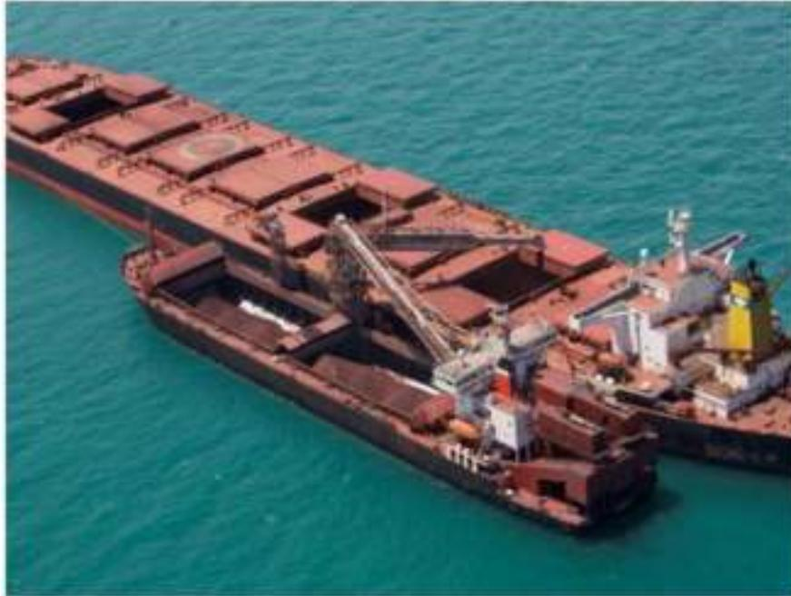
**Figure 10-3 Gravity Transshipment Shuttle Vessel CSL Whyalla transshipping iron ore in South Australia**
