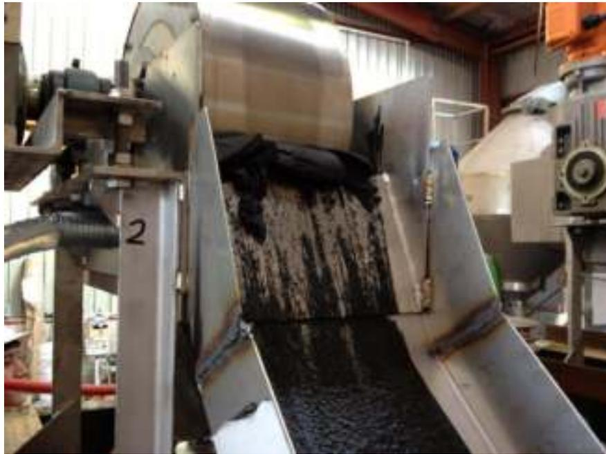
**Figure 7-9 Pilot Plant LIMS-1 Concentrate**
