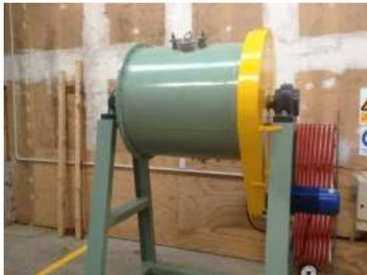
**Figure 7-10 Pilot Plant Ball Mill**
