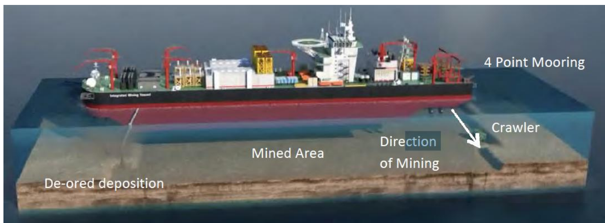
Figure 2: The proposed Integrated Mining Vessel and associated subsurface seabed crawler and simultaneous re-deposition of post processed sands.
